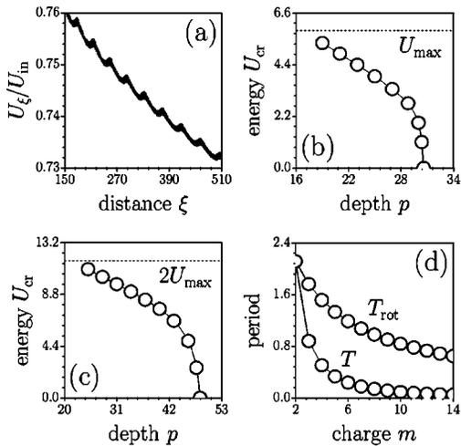
Fig. 4. (a) Energy flow of a single soliton captured by the lattice with  $m=2$  versus propagation distance at  $U_{in}=1.5$  and  $p=32$ . (b) Critical energy versus lattice depth for a single soliton captured by the lattice with  $m=2$  and (c) dipole-mode soliton captured by the lattice with  $m=3$ . (d) Rotation  $T_{rot}$  and self-replication  $T$  periods versus charge  $m$ .
