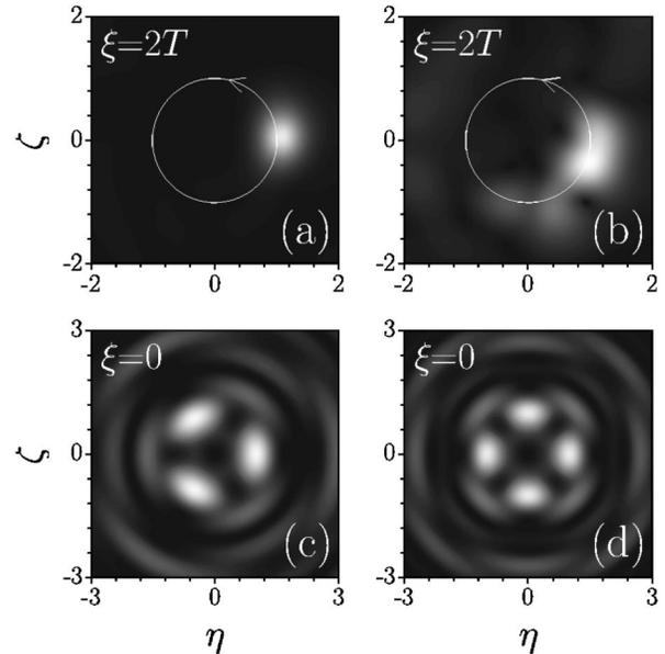
Fig. 3. Output field distributions after two rotations of the lattice with  $m=2$  in (a) nonlinear and (b) linear media at  $U_{\text{in}}=4$  and  $p=25$ . Lattices with (c)  $m=4$  and (d)  $m=5$ .
