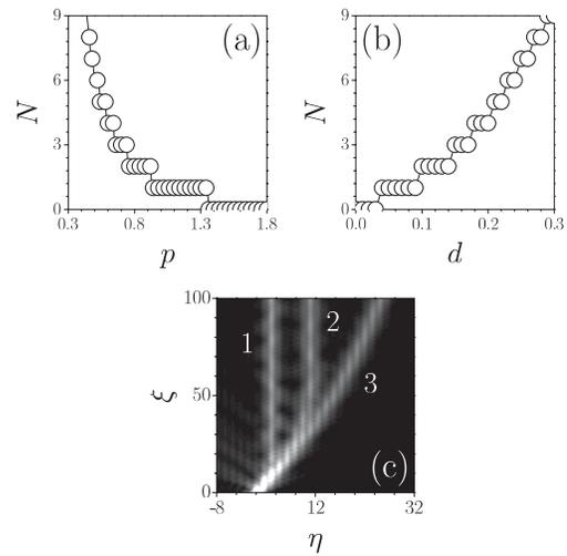
FIG. 4. (a) Output channel number versus lattice depth at  $d = 0.08$ . (b) Output channel number versus nonlocality degree at  $p = 1$ . (c) Soliton propagation trajectories at  $d = 0.1$  (1),  $0.26$  (2), and  $0.4$  (3). Lattice depth  $p = 1$ . In all cases the input soliton form factor  $\chi = 1.2$  and incident angle  $\alpha = 0.5$ .
